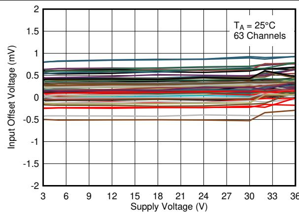
图 6-15. Input Offset Voltage vs. Supply Voltage at 25°C
