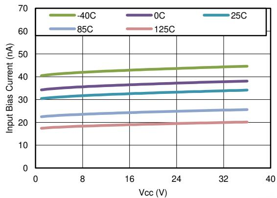
图 6-2. Input Bias Current vs Supply Voltage
