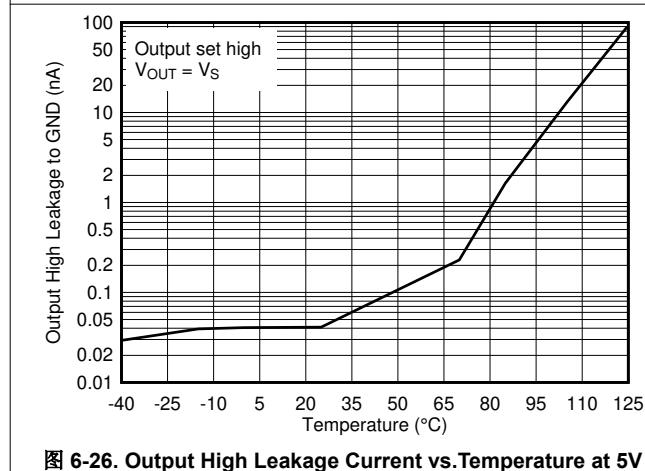
图 6-26. Output High Leakage Current vs. Temperature at 5V
