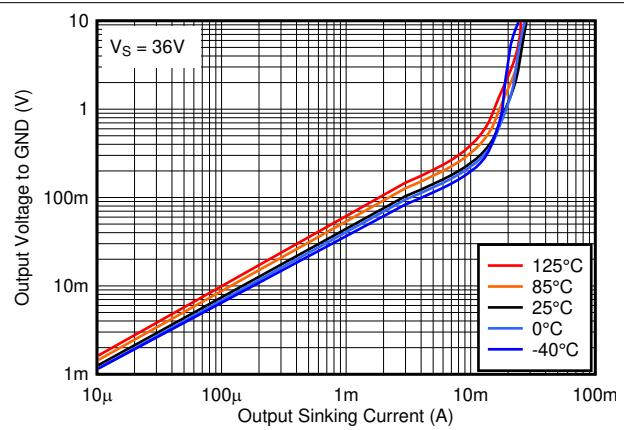
图 6-25. Output Low Voltage vs. Output Sinking Current at 36V
