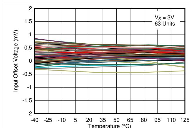
图 6-18. Input Offset Voltage vs. Temperature at 3V
