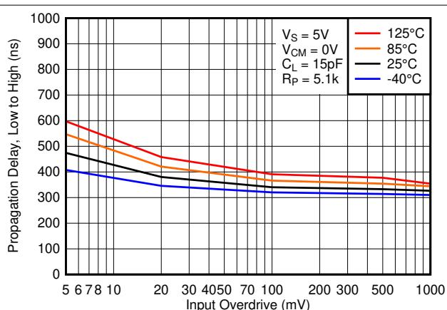
图 6-29. Low to High Propagation Delay vs. Input Overdrive Voltage, 5V
