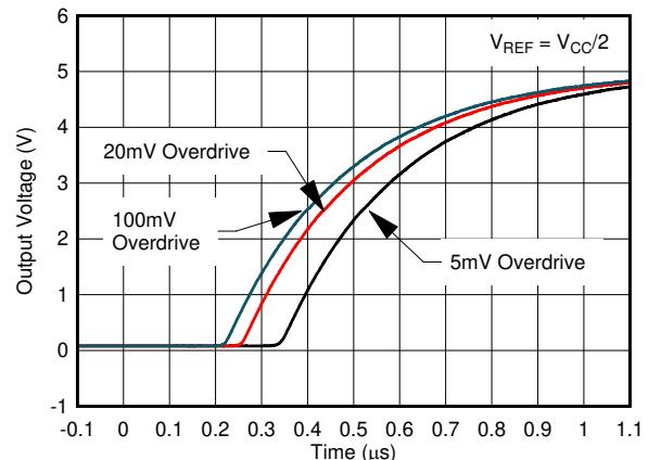
图 6-35. Response Time for Various Overdrives, Low-to-High Transition
