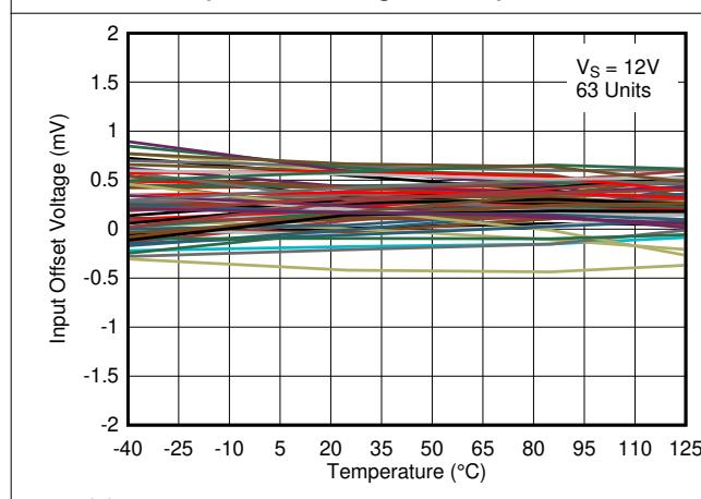
图 6-20. Input Offset Voltage vs. Temperature at 12V
