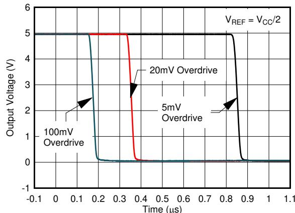
图 6-34. Response Time for Various Overdrives, High-to-Low Transition
