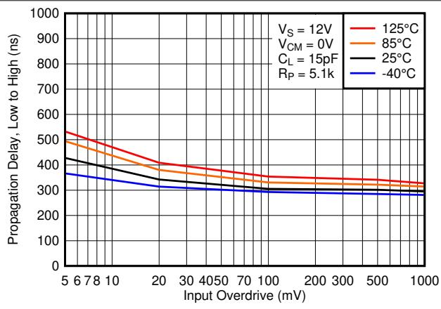
图 6-31. Low to High Propagation Delay vs. Input Overdrive Voltage, 12V
