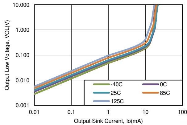
图 6-3. Output Low Voltage vs Output Current ( $I_{OL}$ )
