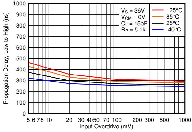
图 6-33. Low to High Propagation Delay vs. Input Overdrive Voltage, 36V
