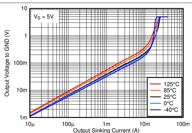
图 6-23. Output Low Voltage vs. Output Sinking Current at 5V
