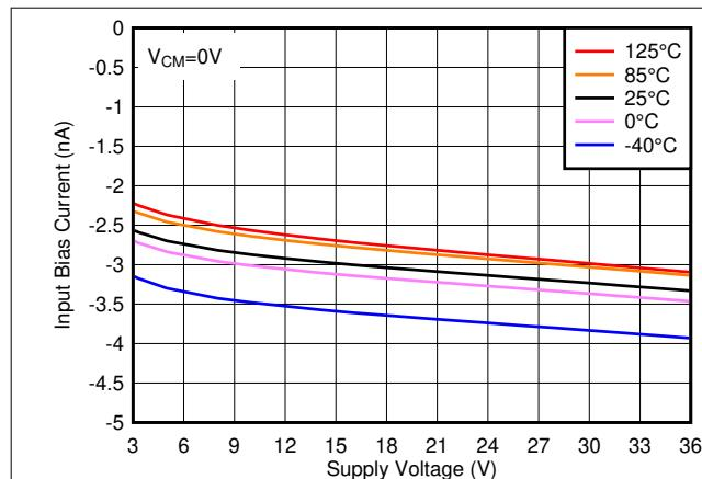
图 6-10. Input Bias Current vs. Supply Voltage
