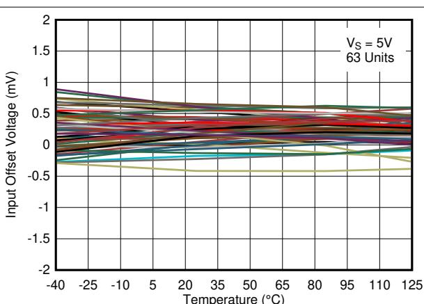
图 6-19. Input Offset Voltage vs. Temperature at 5V
