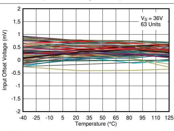
图 6-21. Input Offset Voltage vs. Temperature at 36V
